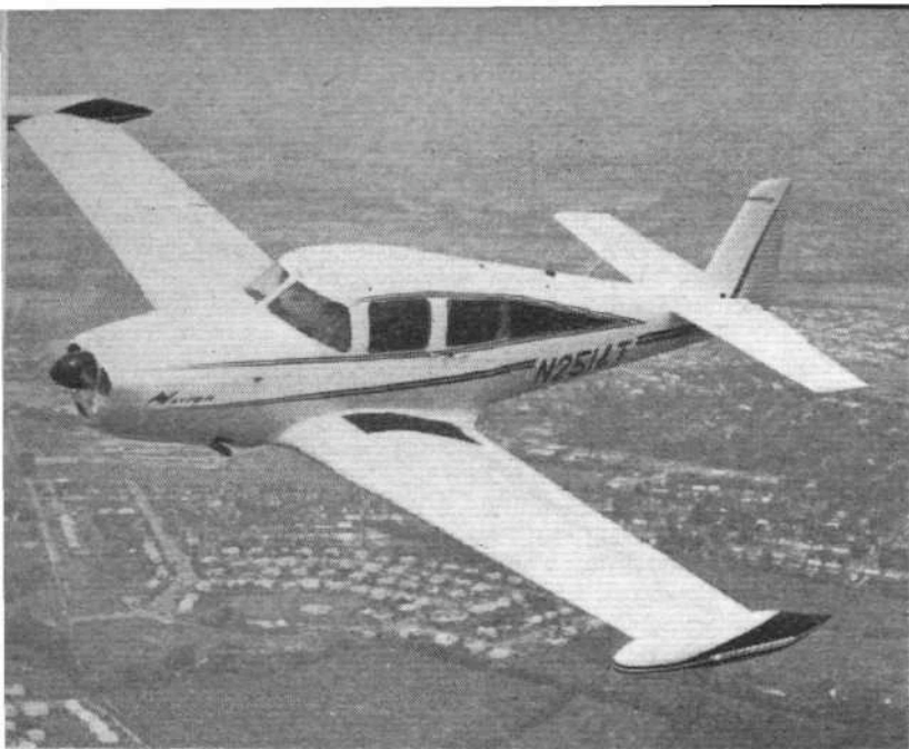
The Navion Aircraft Corporation of Seguin, Texas, is still building the former North American Navion of 20-year-old basic design. The Model H, demonstrated at the recent Reading, Pennsylvania, Show, is in production at the rate of one a week, and 18 have been built. A 285 h.p. Continental IO-520-B powers the five-seater, which has an ex-works basic price of $25,900 (£10,800)
